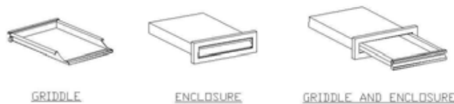
Figure 24. Griddle installation and storage
