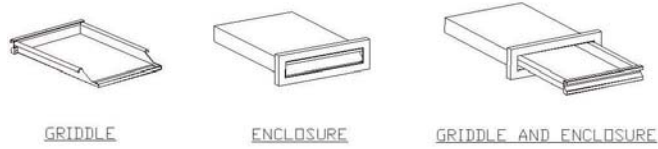
Figure 22. Griddle installation and storage
