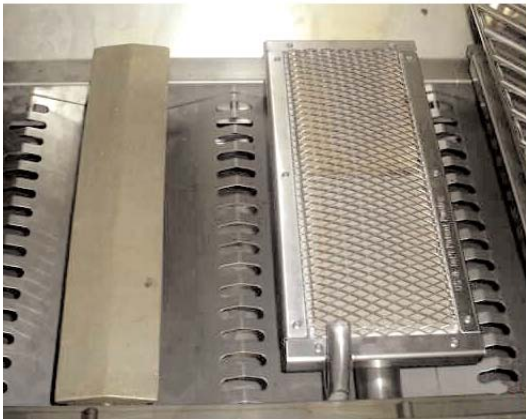
One infrared burner installed
