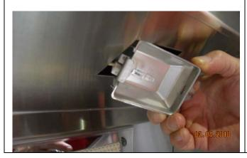
4. Using a small standard screwdriver, remove the one or two white wires from the light socket.
