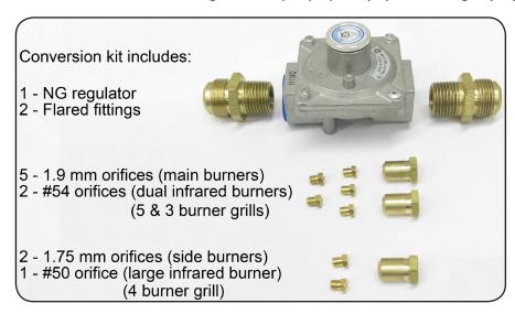
You will need some or all of the fittings (depending on the size of the grill) and the regulator contained in the conversion kit (P/N BBQ07101045). The conversion kit contains orifices to convert five main burners, two small rear infrared burners, one large infrared burner, and two side burners. You will not need all of the parts in the kit.
