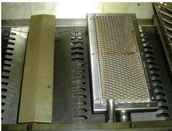
One Sear Zone burner installed
