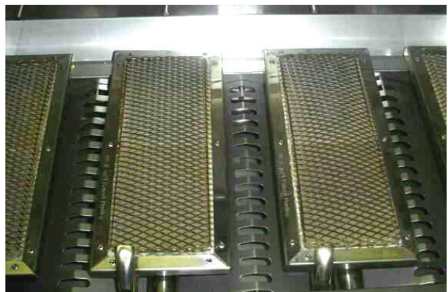
Multiple Sear Zone burners installed
